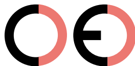
False CE Mark (too far)
